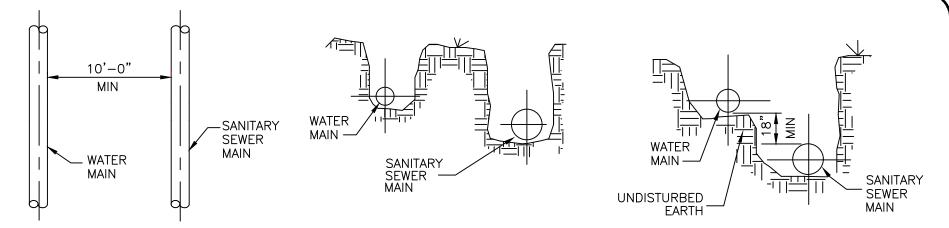
WATER MAINS SHALL BE LAID AT LEAST 10 FEET LATERALLY FROM EXISTING OR PROPOSED SEWERS, UNLESS LOCAL CONDITIONS PREVENT A 10 FOOT LATERAL SEPARATION, IN WHICH CASE:
